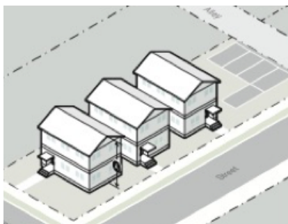
The top image illustrates a property that is in the NL-5: Neighborhood Low Density-5 zone. The diagram on the bottom is taken from the Current Town Land Development Regulations and illustrates allowed development for sites in the NL-5 zone.
